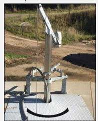
Landia's manure mixer is an allround, efficient, and solid mixer. The low rotation speed makes it very suitable for mixing even very thick manure.
