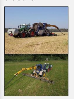
SRS 1200: Slurry is being pumped directly to the machine sparing transportation costs. Low weight means entering fields at an earlier stage
